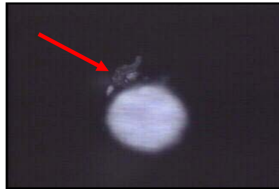
Significantly reduced accumulation of debris on the probe tip after cleaning with 1 µm grit Probe Lap™ .
