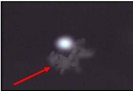
Accumulation of abrasive particles, binder, polyester film and other probing debris on the probe tip after cleaning with 1 µm grit lapping film.
