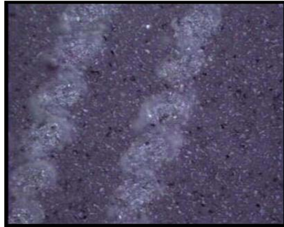
Probe Lap™ – 1 µm grit lapping film after probe cleaning operation at 125°C.
